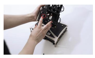
On an 888, the silver mount screws will fit inside this hole.
