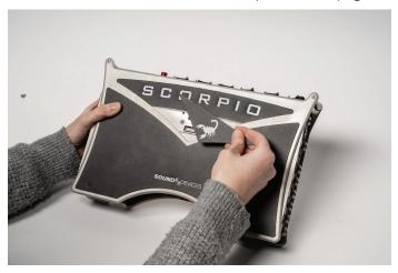
**STEP 2** Using a #4 Phillips Screwdriver, remove the black phillips screw from the Scorpio top panel as shown in the image below. Keep these screws in a safe place as they need to be re-installed if the SL-2 is removed from the Scorpio.
